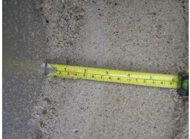
Fig. 16: Measurement of the sand configuration after excavation and JET Master® development
