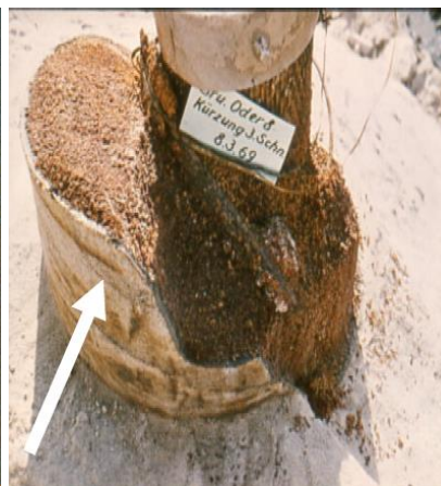
Fig. 2: filter cake is completely existent allowing less water passage
