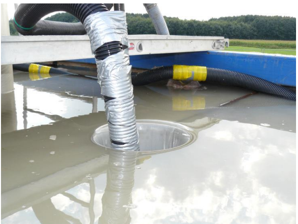
Fig. 15: filled test container with suction device to simulate simultaneous pumping
